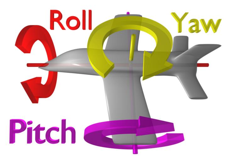
**Figure G.1**: This image illustrates the pitch, roll, and yaw axes of an airplane (which also apply to helicopters). Thanks to Wikipedia contributor ZeroOne for releasing this image under the Creative Commons Attribution 3.0 Unported license.
