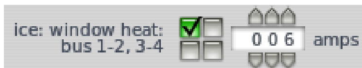
Figure 4.18: A single electrical subsystem, drawing 6 amperes from bus 1
