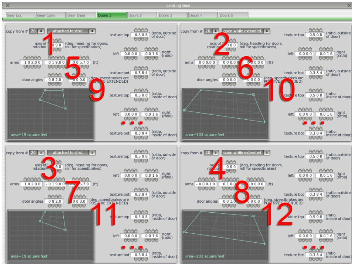
Figure 3.36: Numbering of the landing gear door boxes
