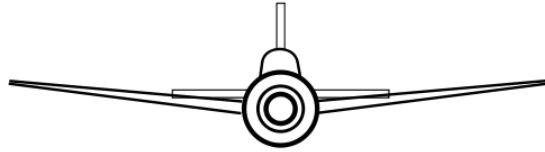
Figure 2: Wing dihedral, the upward angle of the wings, illustrated (thanks to Wikimedia Commons user Steelpillow for the image)
