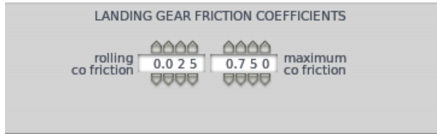
Figure 3.39: The landing gear friction coefficients
