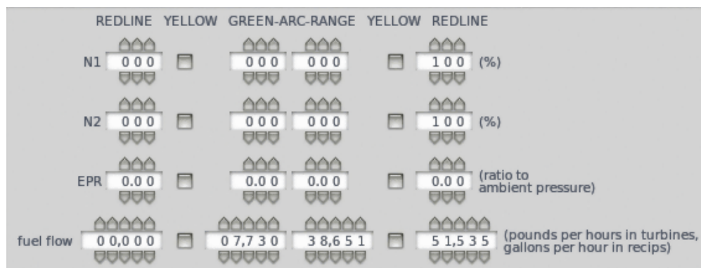
Figure 4.21: The columns for redline, yellow, and green ranges in the Limits tab
