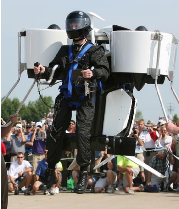
Figure 4.6: The Martin Jetpack, with its ducted fans (thanks to Flickr user martinjetpack for the photo)
