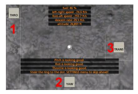
First, there is the throttle control (labeled 1 in the image above). For the descent phases of the mission, this goes from zero to full forward, corresponding to the bottom and top of the screen, respectively. For the command module docking, though, it goes from full backward to full forward, with zero thrust found in the center of its range.
