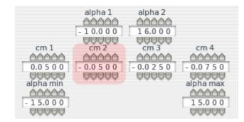
For the NACA 2412, this number is about -0.05, which is a light pitch-down. A wing with a higher camber will have a value of around -0.10, perhaps even -0.13. A symmetrical airfoil will have no pitch tendency at all here, so 0.0 should be entered for that type of airfoil.
