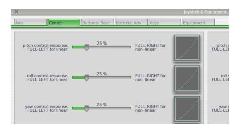
If these three sliders are fully left, then the control response is linear; that is, a 50% stick deflection in the hardware will give 50% control deflection in the aircraft. Likewise, 100% stick deflection in the hardware will give 100% control deflection in the aircraft.
