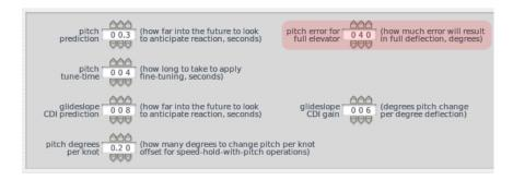
This control is to pitch as the **roll error for full aileron** (from Part A above) control is to roll. It determines how much error between desired and actual pitch is required for full elevator deflection. Remember that the autopilot will automatically reduce the control deflections as the plane speeds up, limiting to maybe 50% control deflection, so it isn't necessary to worry about the system really going to *full* deflection.
