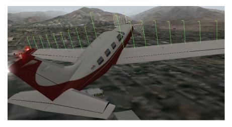
The green bars extending from the wings indicate how much lift each section of the wing is generating; longer bars represent greater force.
