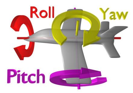
**Pitch**: Movement of the aircraft's nose up or down (see the image above).
