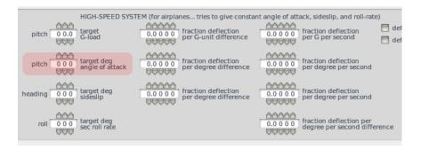
Enter 0.1 for the **fraction deflection per degree difference** (highlighted in the image following), so that if the angle of attack is 10 degrees off, the plane applies full elevator to capture the desired angle of attack.
