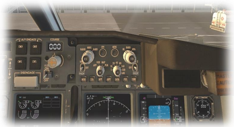
Co-Pilot's EFIS (Electronic Flight Instrument System) Control Panel
