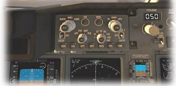
Pilot's EFIS (Electronic Flight Instrument System) Control Panel
