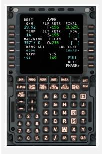
When in PERFORMANCE mode, the MCDU will automatically switch from the DESCENT (DES) Page to the APPROACH (APPR) Page when the deceleration point in the flight plan is reached. Alternatively, the crew may manually activate the approach phase ( see: <a href="Activating Approach Phase">Activating Approach Phase</a>).
