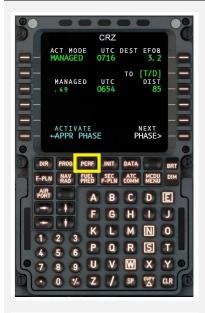
When in PERFORMANCE mode, the MCDU will automatically switch from the CLIMB (CLB) Page to the CRUISE (CRZ) Page when top of climb is reached.
