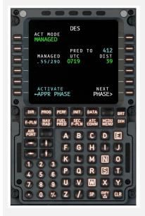
When in PERFORMANCE mode, the MCDU will automatically switch from the CRUISE (CRZ) Page to the DESCENT (DES) Page when top of descent is reached.
