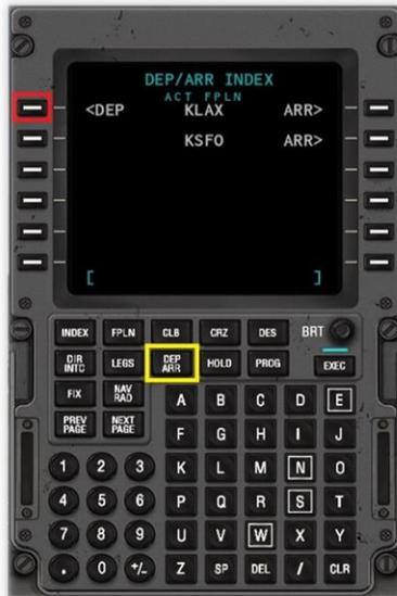
Use the **NEXT PAGE** key to locate the desired runway. In this example, we will be using **25R**.
