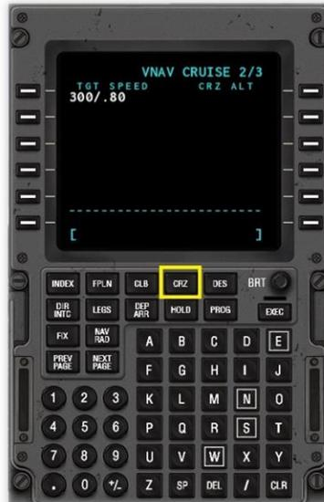
Input the cruise altitude into the scratch pad.
