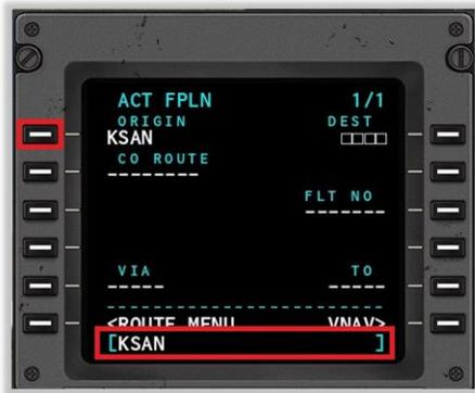
To reset the flight plan, input a new ORIGIN into the 'Scratch Pad'.
