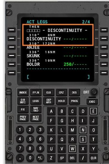
To repair the discontinuity, the missing waypoints **BSR** and **CARME** must be re-introduced into our flight plan, at the correct locations.
