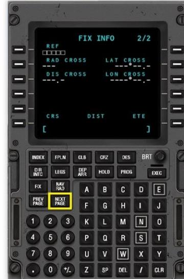
Input the name of the navigation aid that defines the fix. This is the Woodside VOR, which has the identifier **OSI**.
