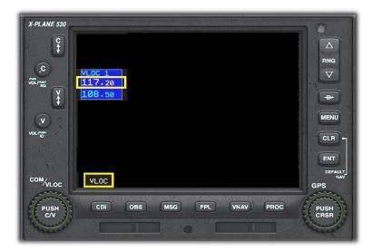
Using your primary navigation radio (in this example the GNS 530), select the desired VOR frequency.
