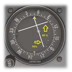
If the virtual glideslope tracking does not arm automatically, the pilot may force this to occur manually – after satisfying the 50% / 60% rules for glideslope arming outlined above. Push the ALT button to engage ALTITUDE HOLD and GLIDESLOPE modes concurrently. When the glideslope is captured, ALTTITUDE mode will cancel automatically, and the autopilot will track the glideslope.
