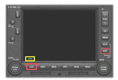
With a flight plan programmed into your GPS device (in this example the GNS 530), select GPS mode.
