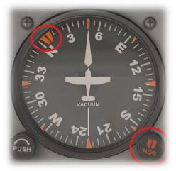
The autopilot is not connected to the OBS ring of your VOR instrument, and therefore it is necessary to also select the desired radial using the Directional Gyro (DG) Heading (HDG) rotary.
