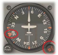
Using the HDG (Heading) bug, manually select the desired intercept course.
