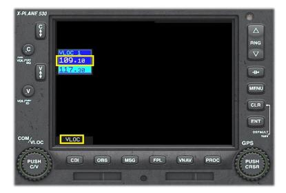
Using your primary navigation radio (in this example the GNS 530), select the desired ILS frequency.
