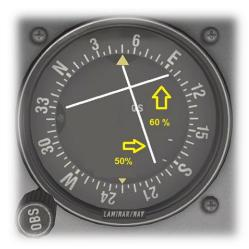
If glideslope tracking does not arm automatically, the pilot may force this to occur manually – after satisfying the 50% / 60% rules for glideslope arming outlined above. Push the ALT button to engage ALTITUDE HOLD and GLIDESLOPE modes concurrently.
