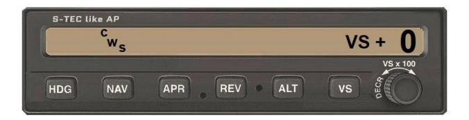
In this mode, the autopilot suspends control of the aileron and trim servos, allowing the pilot to provide the desired input via the control column.
