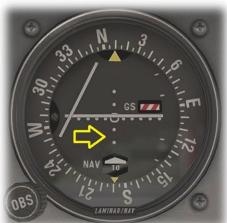
When the Course Deviation Indicator on the VOR instrument is centered, the aircraft is on the desired radial, and the autopilot will maintain that situation.
