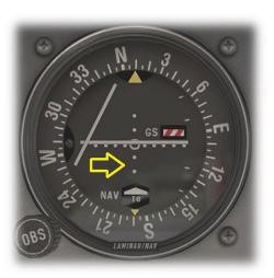
As soon as the HDG mode indication vanishes from the display, the pilot must alter the HDG (Heading) bug to the desired front-course to the VOR (unless the aircraft is equipped with an HSI).
