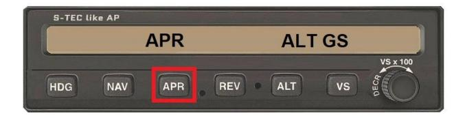
For the virtual glideslope tracking to arm automatically when the pilot initiates APR (Approach) mode, the localizer deflection must be no more than 50% of maximum, the aircraft must be under the glideslope, and the glideslope deflection must be at least 60% of maximum.
